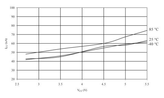
Figure 31-51. Programming Current vs. V<sub>CC</sub>
