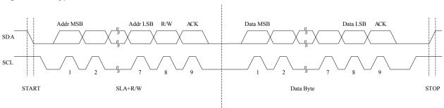
Figure 24-7. Typical Data Transmission
