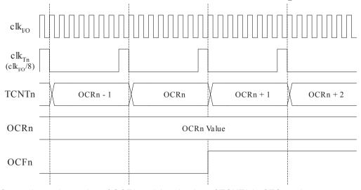
The next figure shows the setting of OCF0 and the clearing of TCNT0 in CTC mode.
