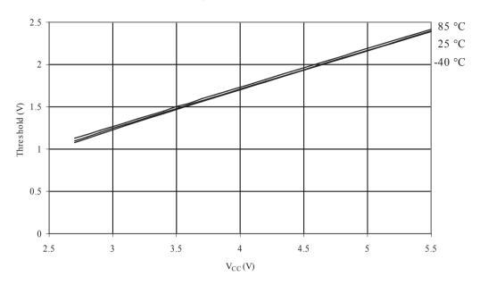
Figure 31-27. I/O Pin Input Hysteresis vs.  $V_{\text{CC}}$
