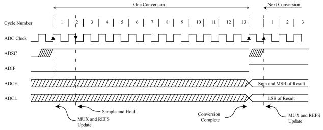
Figure 26-6. ADC Timing Diagram, Auto Triggered Conversion
