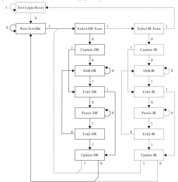
Figure 29-15. State Machine Sequence for Changing/Reading the Data Word
