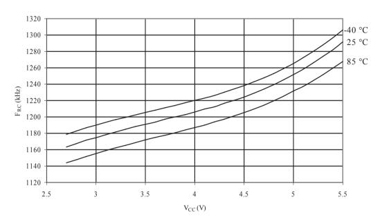
Figure 31-35. Calibrated 8MHz RC Oscillator Frequency vs. Temperature
