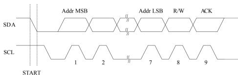
Figure 24-5. Address Packet Format
