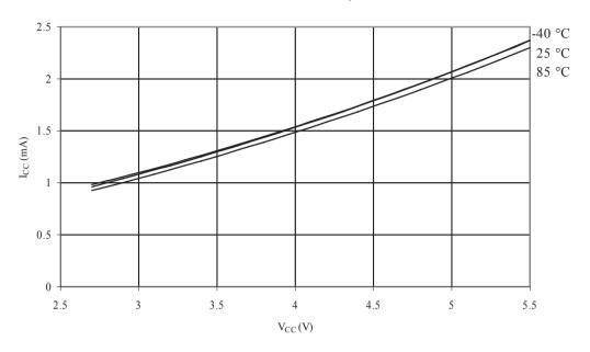
Figure 31-11. Idle Supply Current vs. VCC (Internal RC Oscillator, 1MHz)
