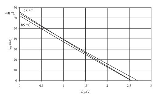
Figure 31-19. Reset Pull-up Resistor Current vs. Reset Pin Voltage (VCC = 5V)
