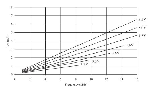
Figure 31-9. Idle Supply Current vs. VCC (Internal RC Oscillator, 8 MHz)
