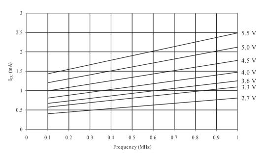
Figure 31-53. Reset Supply Current vs. Frequency (1 - 16MHz, Excluding Current Through The Reset Pull-up)
