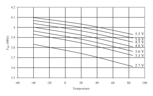
Figure 31-39. Calibrated 4MHz RC Oscillator Frequency vs.  $V_{\text{CC}}$
