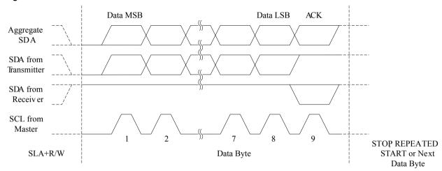
Figure 24-6. Data Packet Format
