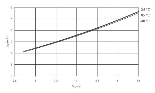
Figure 31-5. Active Supply Current vs. VCC (Internal RC Oscillator, 1MHz)
