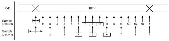
The decision of the logic level of the received bit is taken by doing a majority voting of the logic value to the three samples in the center of the received bit. The center samples are emphasized on the figure by
