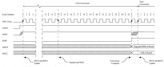
Figure 26-5. ADC Timing Diagram, Single Conversion
