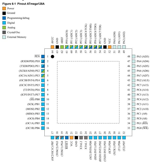
**Note:** The Pinout figure applies to both TQFP and MLF packages. The bottom pad under the QFN/MLF package should be soldered to ground.
