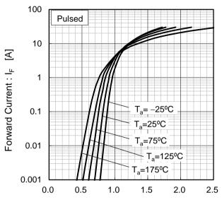
Fig.2 V<sub>F</sub> - I<sub>F</sub> Characteristics
