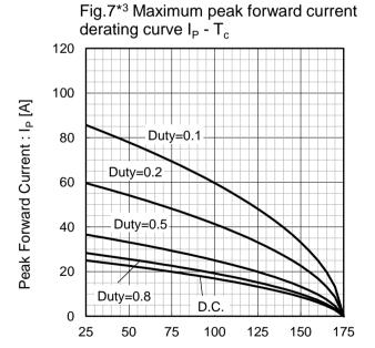
Case Temperature :  $T_c$  [°C] \*3 Based on max Vf, max  $R_{th(j-c)}$  Valid for switching of above 10kHz, excluding D.C. curve.
