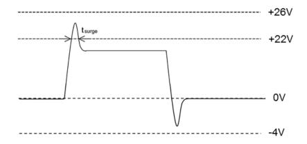
Please note especially when using driver source that  $V_{\text{GSS}\_surge}$  must be in the range of absolute maximum rating.
