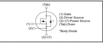
Please note Driver Source and Power Source are not exchangeable. Their exchange might lead to malfunction.
