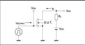
Fig.2-1 Switching Characteristics Measurement Circuit
