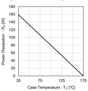
Fig.1 Power Dissipation Derating Curve
