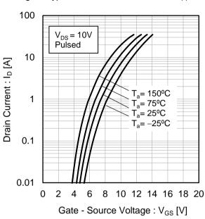
Fig.11 Typical Transfer Characteristics (I)
