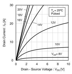
Fig.4 Typical Output Characteristics(I)
