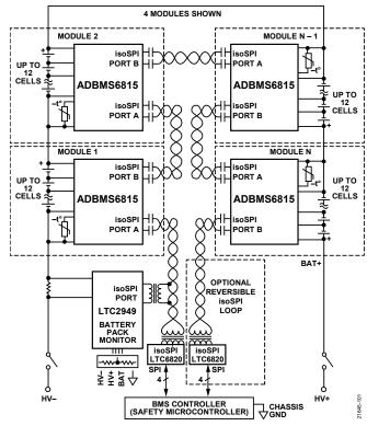
Figure 1. Typical Application Circuit
