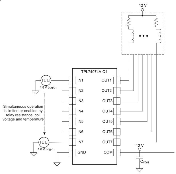
Figure 7. Inductive Load Driver Schematic
