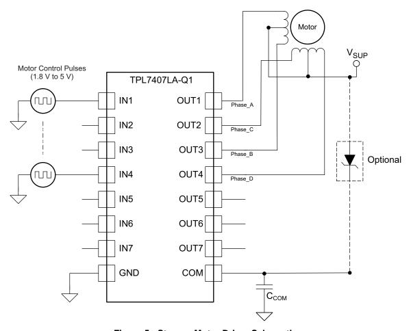
Figure 5. Stepper Motor Driver Schematic
