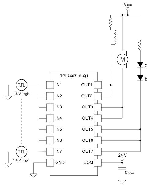
Figure 6. Multi-Purpose Sink Driver Schematic
