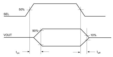
Figure 1. Select to Switch  $t_{ON}$  and  $t_{OFF}$
