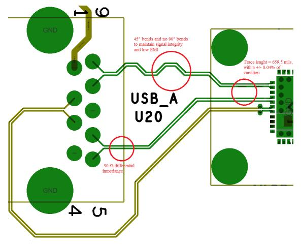
Figure 11. USB Signals Routing Example
