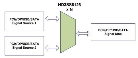
Figure 6. Two Signal Sources to One Destination
