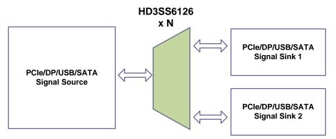
Figure 7. One Signal Sources to Two Destination
