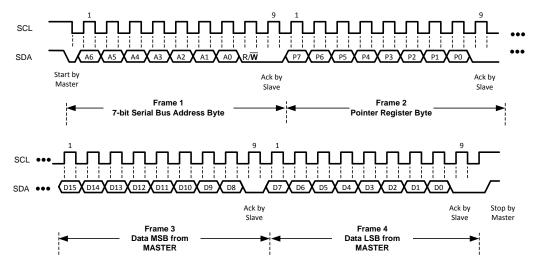
Figure 10. Writing Frame (Configuration Register)
