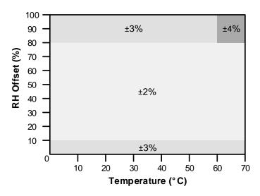
Figure 17. Relative Humidity Accuracy vs Temperature
