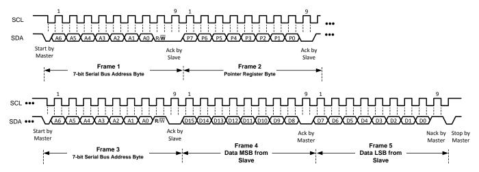
Figure 11. Reading Frame (Configuration Register)
