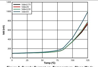
Figure 9. Supply Current vs. Temperature, Sleep Mode
