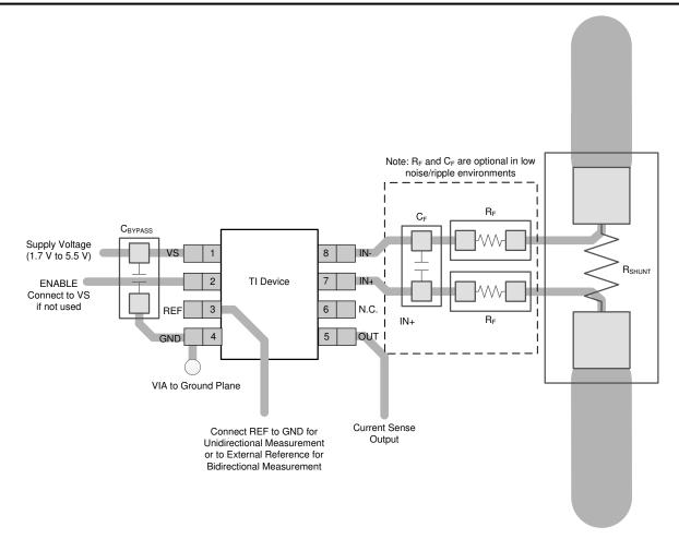
Figure 10-2. Recommended Layout for SOT-23 (DDF) Package
