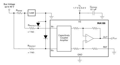
Figure 8-4. Transient Protection Using Dual Zener Diodes
