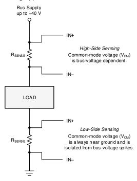
Figure 7-1. High-Side and Low-Side Sensing Connections
