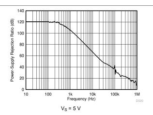
Figure 6-2. Power-Supply Rejection Ratio vs. Frequency
