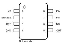
Figure 5-3. DDF Package 8-Pin SOT-23 Top View
