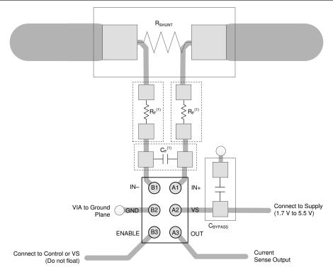
Figure 10-3. Recommended Layout DSBGA (YFD) Package
