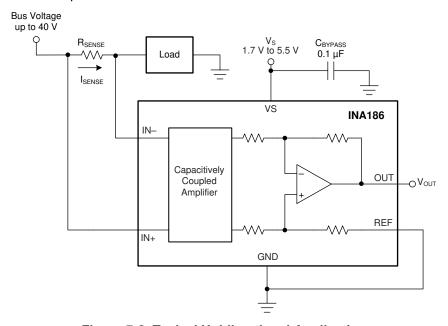
Figure 7-2. Typical Unidirectional Application
