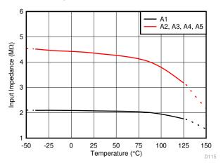
Figure 8-3. Differential Input Impedance vs. Temperature
