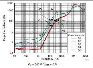
Figure 6-24. Output Impedance vs. Frequency
