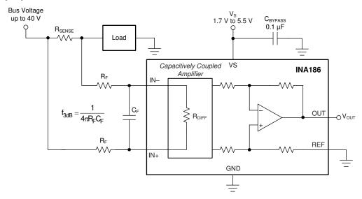
Figure 8-2. Filter at the Input Pins
