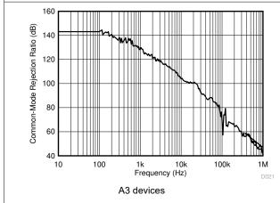
Figure 6-3. Common-Mode Rejection Ratio vs. Frequency
